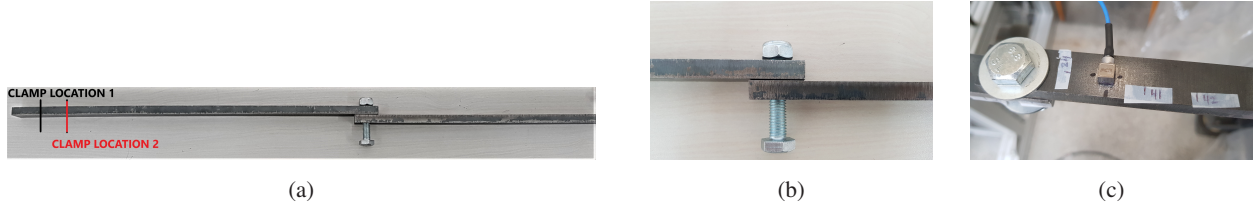
Figure 1: The experimental set-up of the beam measurements. (a) the beam structure with part A (left) attached to part B (right). The picture also shows the different clamping locations. (b) a close-up of the bolted joint unattached. (c) The beam in the setup with one of the PCB tri-axial sensors.
